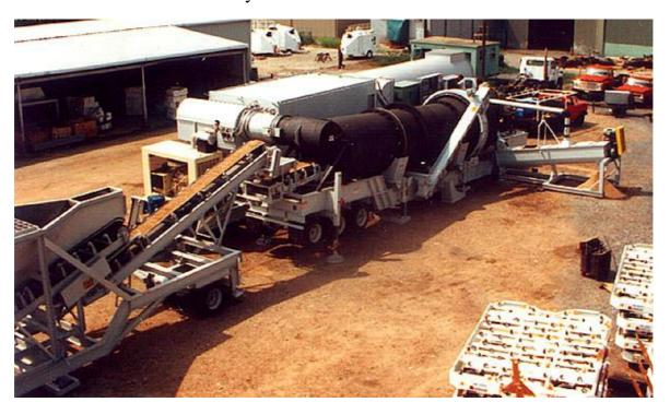
7.0' diameter dryer soil remediation plant, light oil contaminated soil
