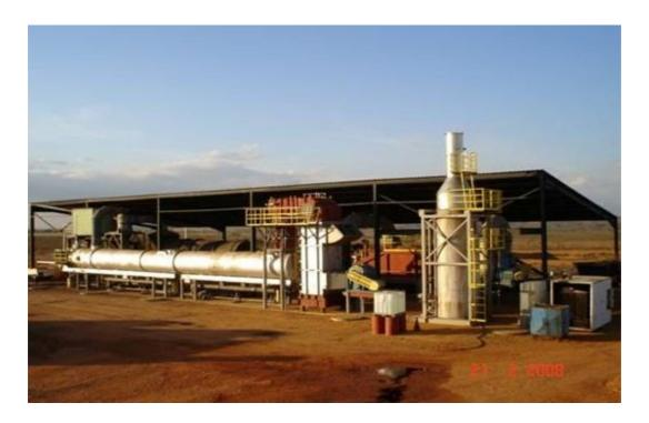
Used 15 ton per hour thermal soil plant built for heavy hydrocarbon. Plant includes single cold feed bin, weigh conveyor with belt scale, 6' x 30' counter flow with dust collar and hauck oil burner, single unit with return augers to dryer, and an oxidizer with a four-second Retention Time, Burner and Fines Removal.
