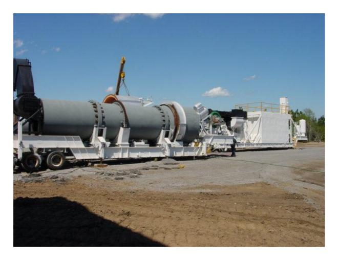
7.0' Diameter Dryer Soil Remediation Plant, Heavy Oil Contaminated Soil
