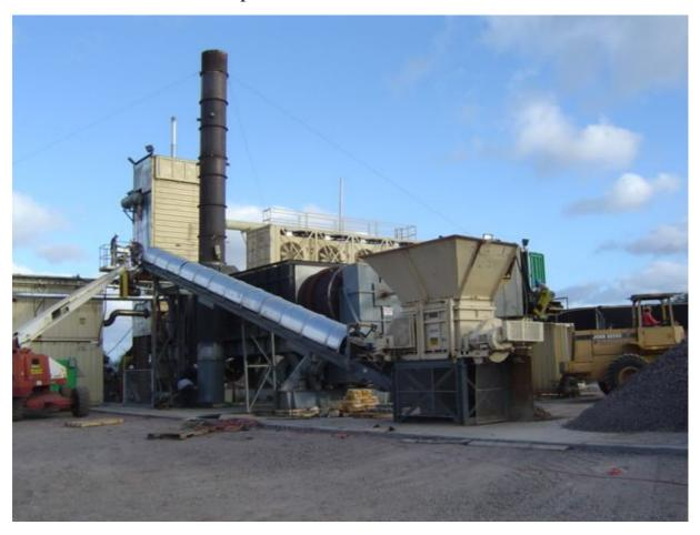
7.0' Indirect Fired Dryer, Triple Shell, Gas Condensing System
