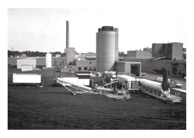
7.0' diameter dryer soil remediation plant, heavy oil contaminated soil
