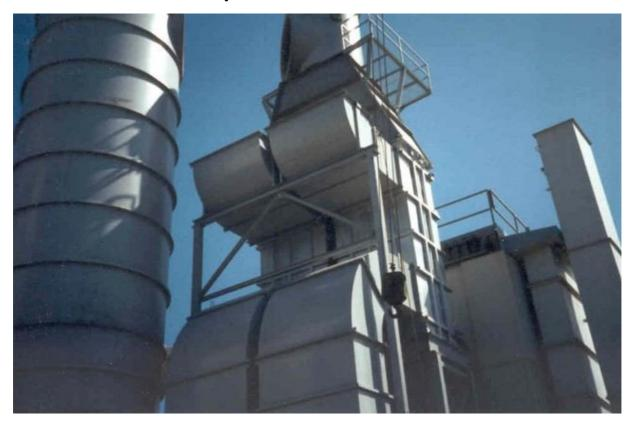
7.0' Diameter Dryer Soil Remediation Plant, Light Oil Contaminated Soil
