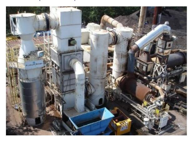
Remediation of 34,000 tons of hydrocarbon contaminated soils using mobile Thermal Desorption Technology.
