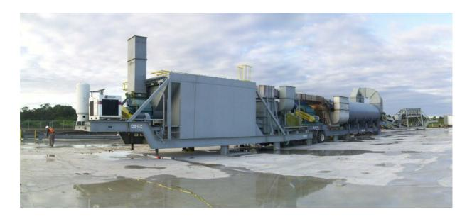
Super 7' diameter dryer soil remediation plant, heavy oil contaminated soil capable, chlorine and sulfur gas reduction equipment
