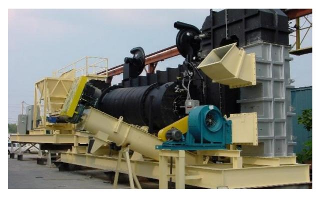
4.5' diameter dryer soil remediation plant, heavy oil contaminated soil capable. feed bin, dryer, and soil conditioner on first load. oxidizer, heat exchanger, baghouse on second load. highly portable
