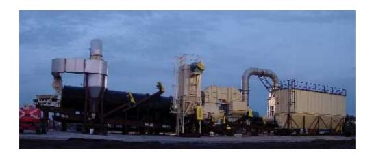
Super 7' Diameter Dryer Soil Remediation Plant, Heavy Oil Contaminated Soil Capable, Chlorine and Sulfur gas Reduction Equipment
