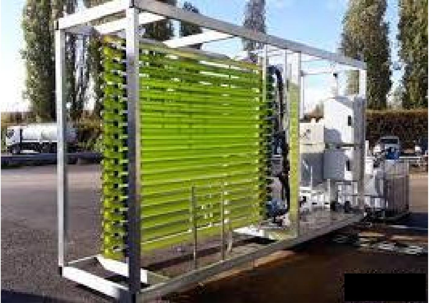
The Tubular Spirulina Algae Bioreactors model EP.SPIRU 400 &700 are built on one standard 40” container frame containing the Cultivation and Preparation Equipment. Models 800 & 1200 are built on two standard 20” &40 containers frames.
