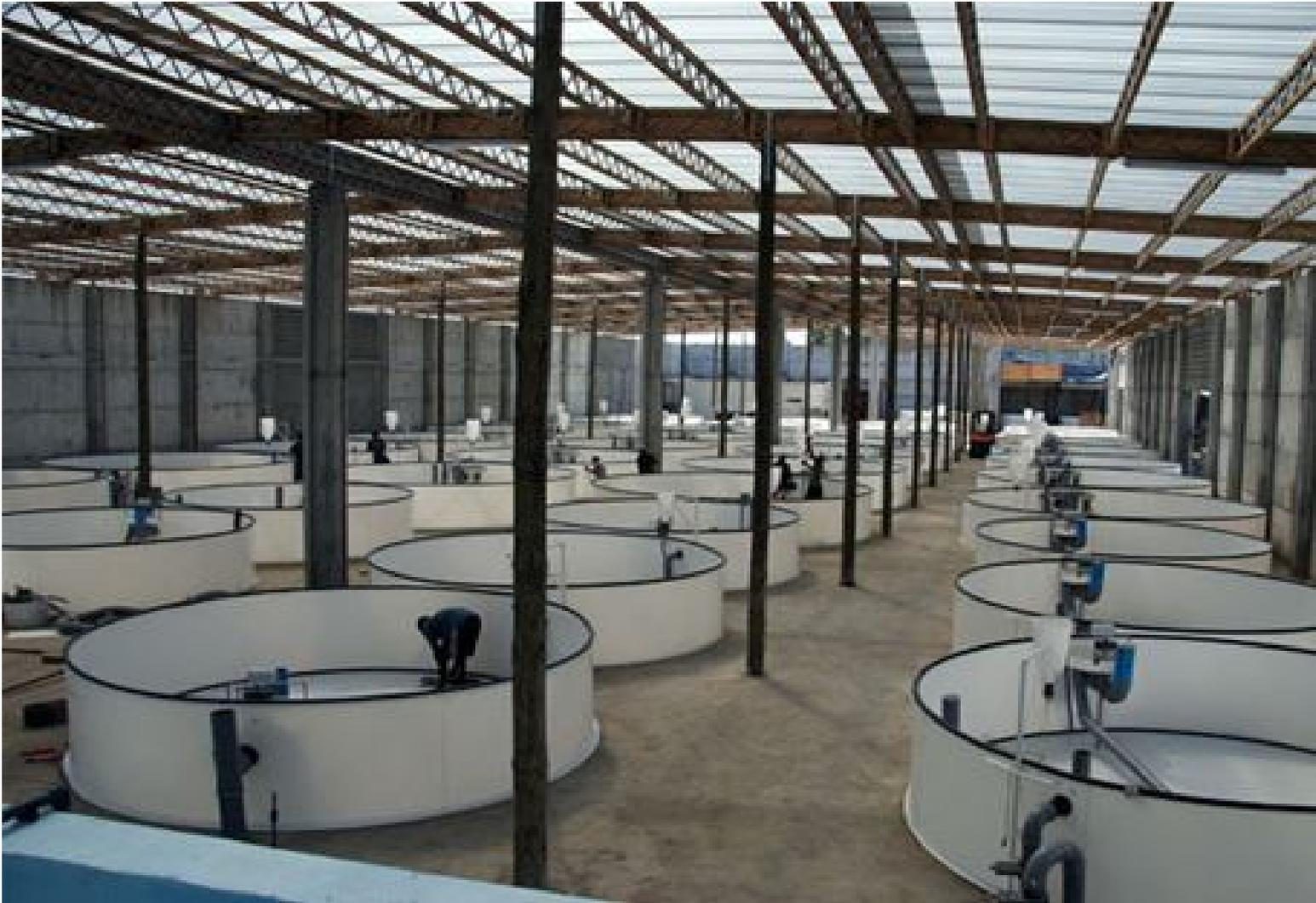
The Tankage Spirulina Algae Bioreactors, EP.SIRU are built either in transparent or opaque polyethylene tanks for above ground installation. Optional underground installation in opaque tanks is available. Central gathering, treatment and drying station is normally centralized in the plant.
