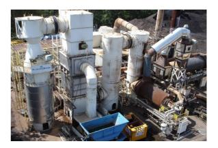
contaminated material were excavated to depths of up to 14 feet. Materials greater than 2 inches in diameter were removed before placing the soil in the desorber and heating it to 900°F. About 225 tons of contaminated soil were treated each day. A small amount of treated soil had to be placed back in the desorber a second time to meet cleanup goals for PCBs, SVOCs, and arsenic. The cleaned soil was used to backfill the areas that had been excavated.
