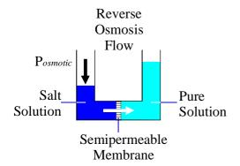
In practice, the RO devices are cross flow filtration where the feed stream is split into permeate(pure) and brine (concentrate/reject) streams. The cross flow configuration allows for continuous duty process as the concentrate sweeps away the membrane 's rejected salts and discharge them to the brine stream.
