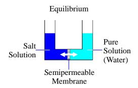
The osmosis process is reversible. By applying osmotic pressure on salt solution side, water can pass through semi-permeable membrane to the pure water side leaving salts behind. This is called reverse osmosis RO process. The RO process is widely used in water desalination. t
