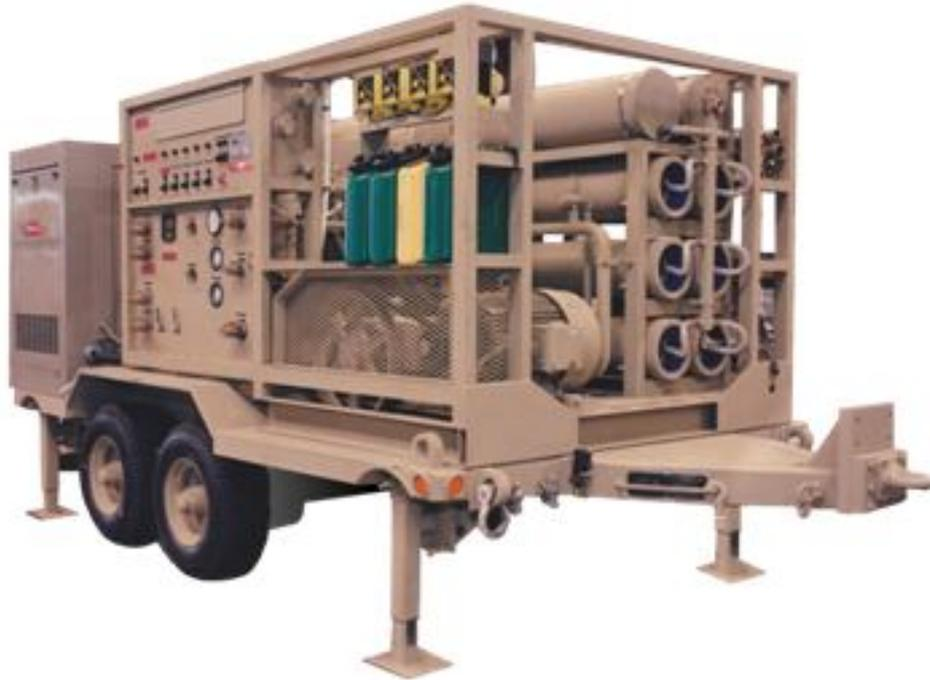
EPECO is manufacturing ROWPU's, the Reverse Osmosis Water Purification Units, for battle field operations.
