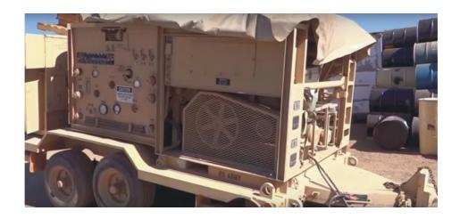
Each Gulf War II EP.ROWPU unit were capable of producing up to 272 cubic meters per day from brackish water or 160 cubic meters per day from seawater sources. **EP.ROWPU** units can be equipped with NBC (Nuclear, Biological and Chemical ) de-contaminators which can secure the production of pure water under the most difficult military operations conditions.
