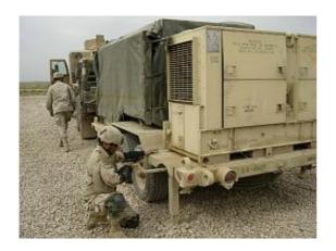
EP.ROWPU's are manufactured at a wide capacity range (50-250 cubic meters per day). Standard EP.ROWPU's for land based operations are built for installation on a rough terrain military truck for full mobility. The basic EP.ROWPU skid can be easily detached for static installation.
