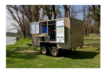
EP.ROWPU, the Reverse Osmosis Water Purification systems, designed to provide purified drinking water to soldiers in battle fields. EP.ROWPU can convert contaminated swamps, wells, rivers or oceans water into fresh drinking water within 2 hours from deployment.
