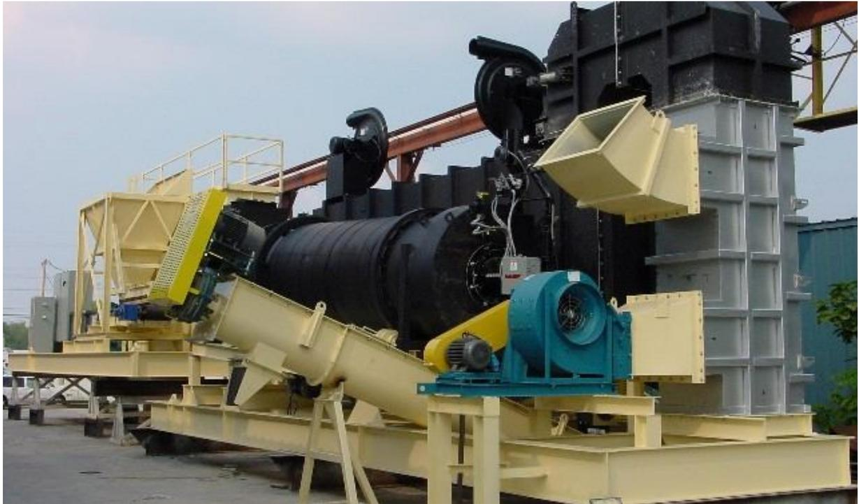
4.5' diameter dryer soil remediation plant, heavy oil contaminated soil capable. feed bin, dryer, and soil conditioner on first load. oxidizer, heat exchanger, baghouse on second load. highly portable
