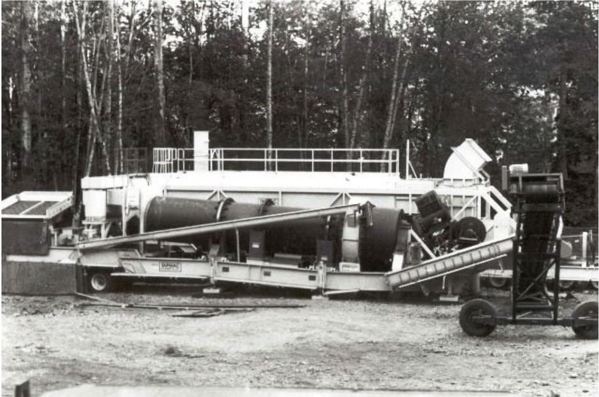
5.5' Diameter Dryer Soil Remediation Plant, Heavy Oil Contaminated Soil Capable. Feed Bin, Dryer, And Soil Conditioner On First Load. Oxidizer, Heat Exchanger, Baghouse On Second Load. Highly Portable
