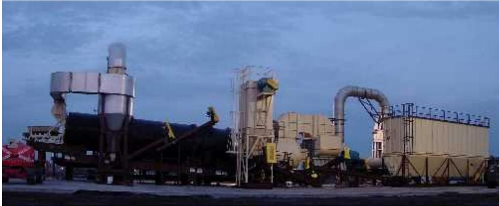
Super 7' Diameter Dryer Soil Remediation Plant, Heavy Oil Contaminated Soil Capable, Chlorine and Sulfur gas Reduction Equipment
