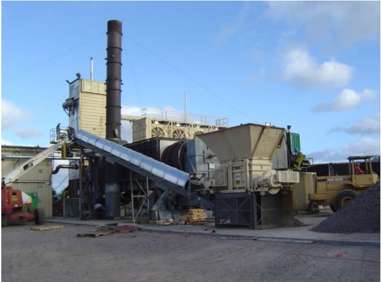
7.0' Indirect Fired Dryer, Triple Shell, Gas Condensing System
