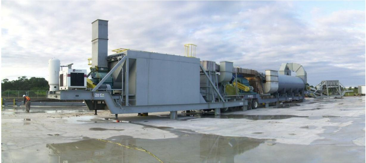
Super 7' diameter dryer soil remediation plant, heavy oil contaminated soil capable, chlorine and sulfur gas reduction equipment
