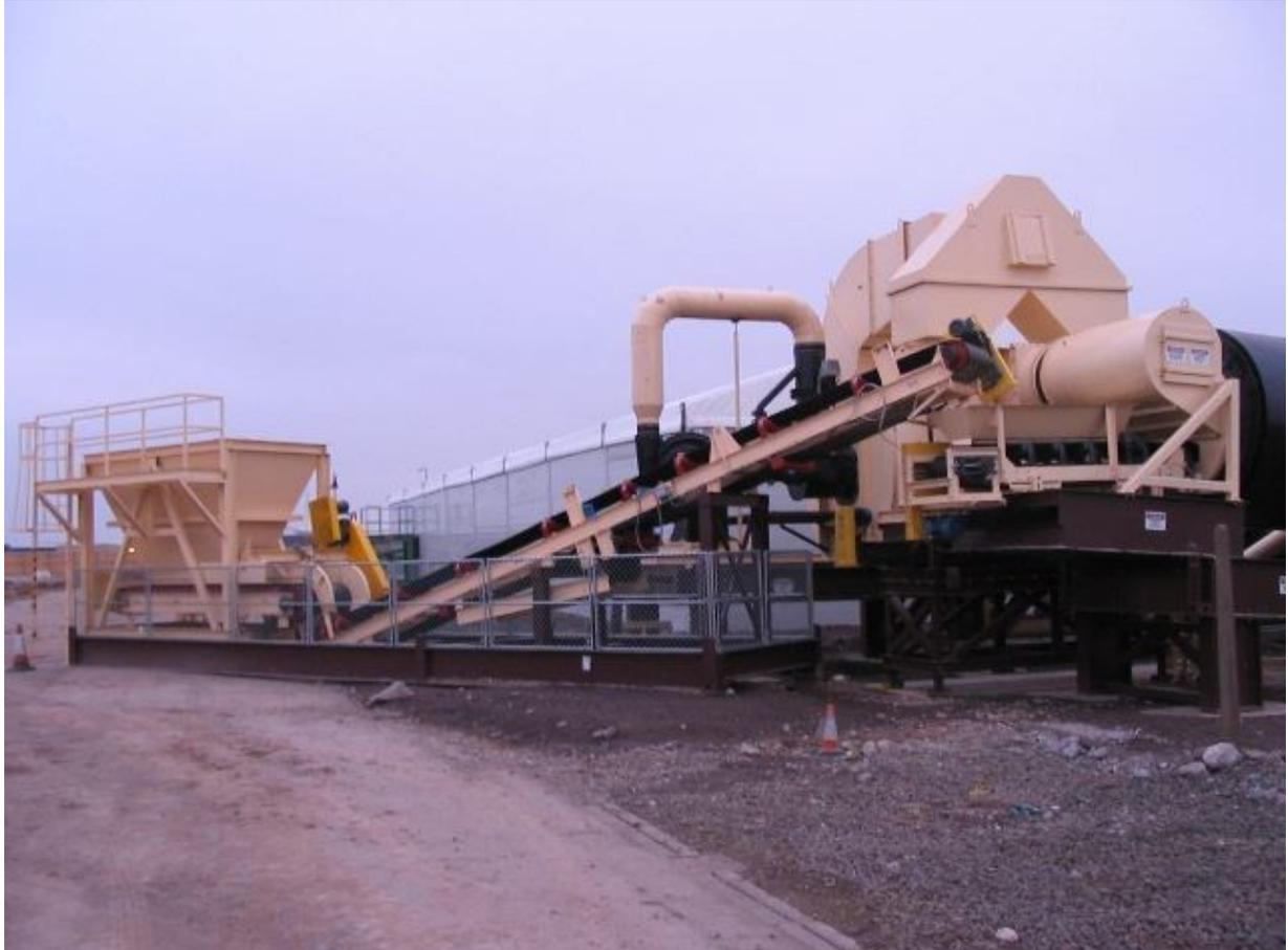
Super 7' Diameter Dryer Soil Remediation Plant, Heavy Oil Contaminated Soil Capable, Chlorine and Sulfur gas Reduction Equipment
