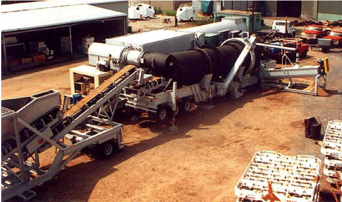
7.0' diameter dryer soil remediation plant, light oil contaminated soil
