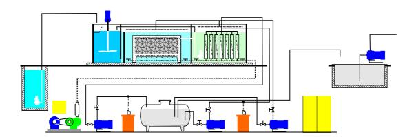
The phase [I] biological reactor is working on the Fixed Film Contractors **FFC** principle. The **FFC** Biological Reactor is an aerobic activated sludge wastewater treatment compartment where **FFC** provide a bed to support the biomass film that digests the bio-degradable waste material in the wastewater.
